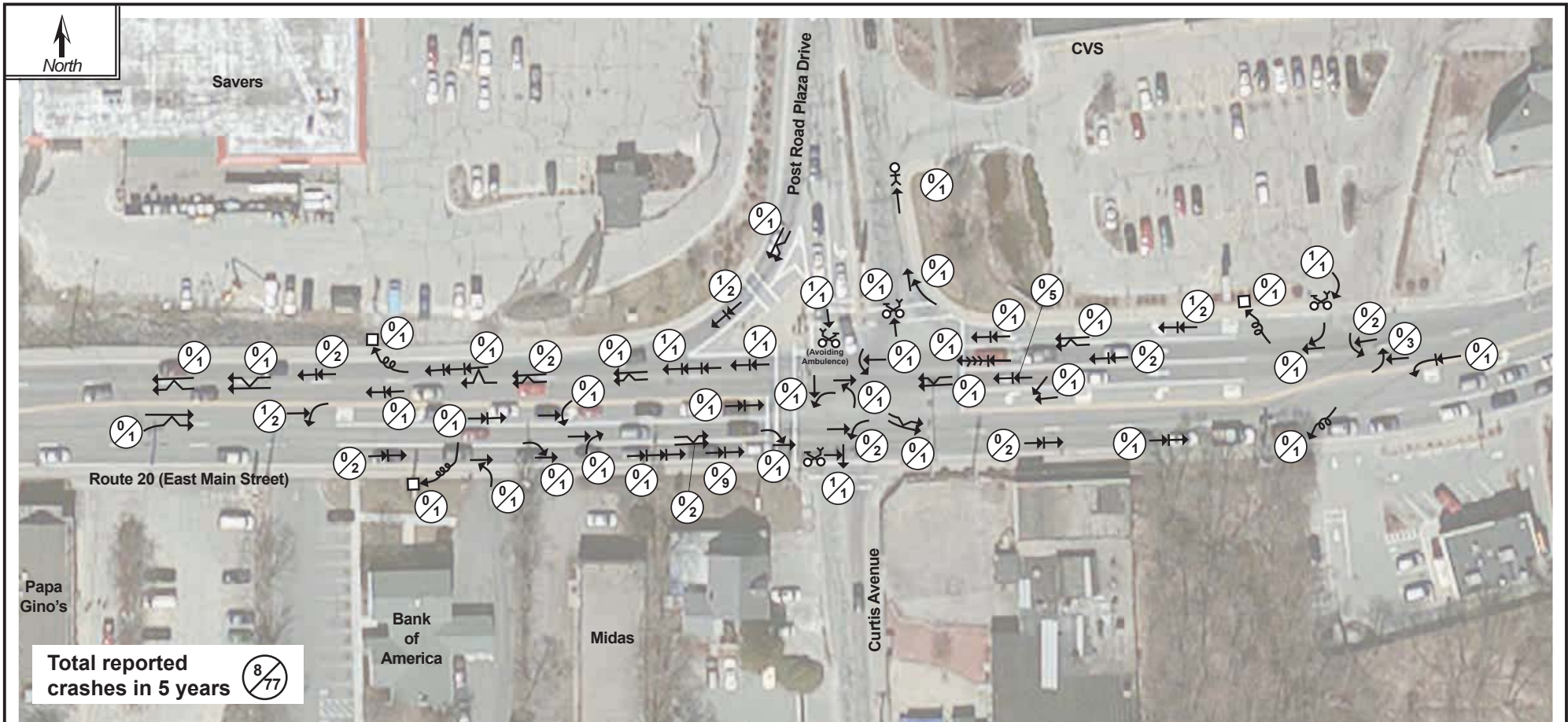
Figure H-6 Collision Diagram: Route 20 at Curtis Avenue Marlborough Police Reports: January 2011–December 2015
