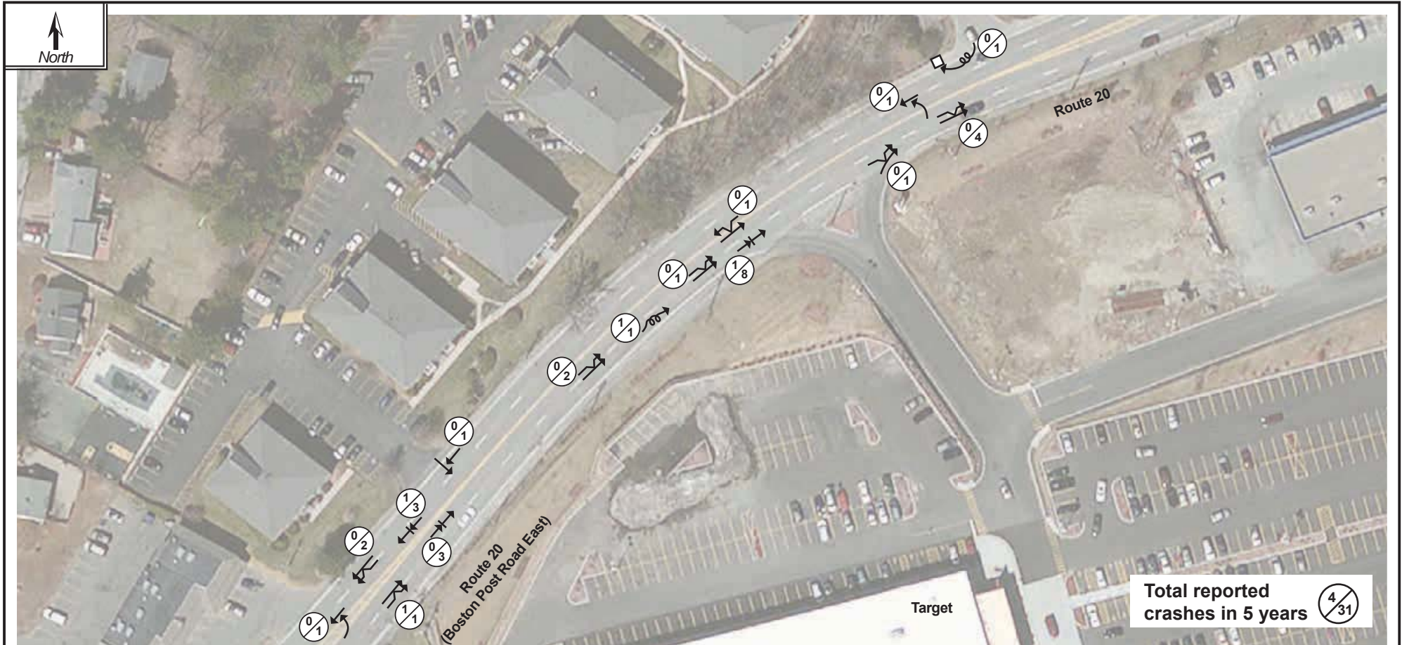
Figure H-13 Collision Diagram: Route 20 between Farm Road and Dicenzo Boulevard Marlborough Police Reports: January 2011–December 2015
