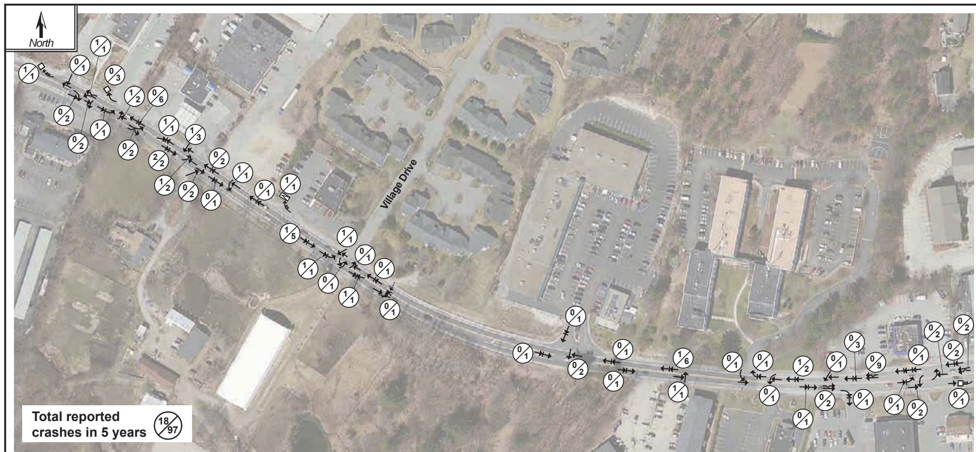
Figure H-11 Collision Diagram: Route 20 between Victoria Lane and Farm Road Marlborough Police Reports: January 2011–December 2015
