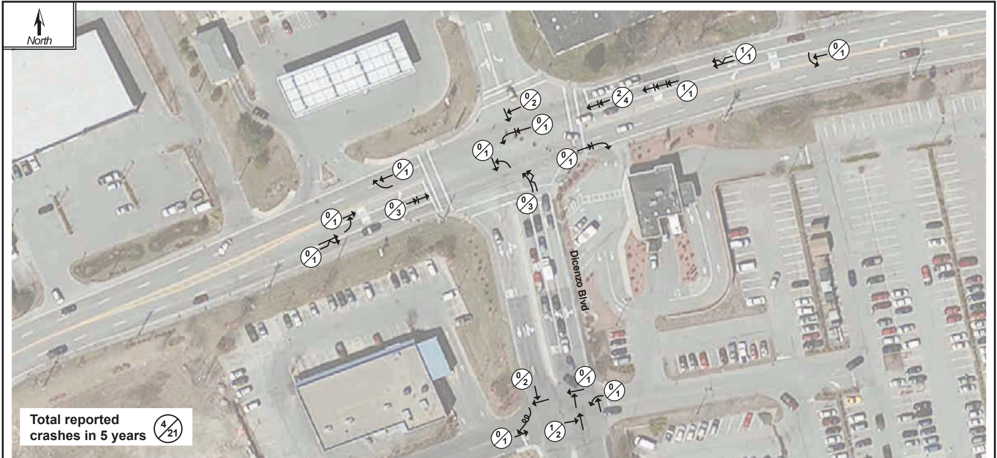
Figure H-14 Collision Diagram: Route 20 at Dicenzo Boulevard Marlborough Police Reports: January 2011–December 2015
